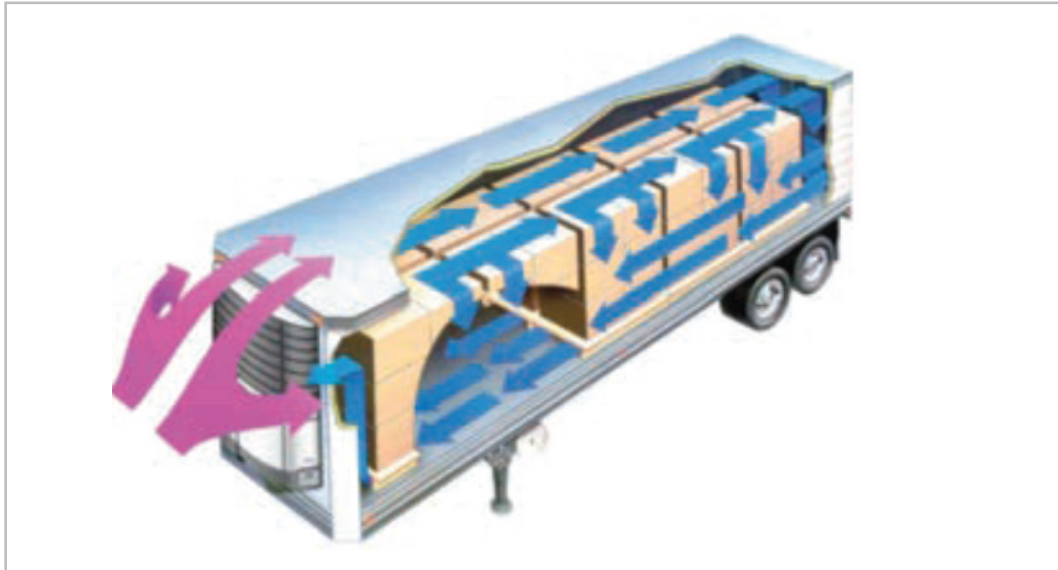
Fig 5: Uniform air circulation in a reefer truck
